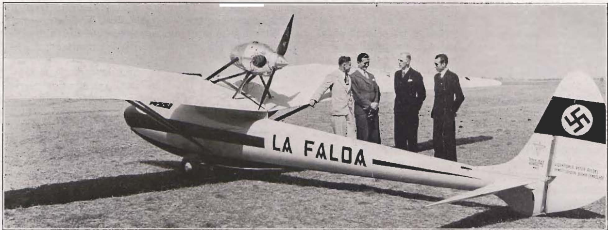
The "Motor Condor," a sailplane with a small motor which can be fixed on for temporary use by means of four bolts. Peter Riedel, the pilot, is second from the left.
